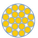
Glued fiber bundles always feature blind spots between individual fibers. That results in a loss of the light input between 25 and 50 percent.
