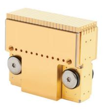
Lasertel's fluid cooled laser diode arrays utilize a patented monolithic design that requires only filtered water (not deionized). This eliminates the most common failure mechanisms associated with microchannel cooled laser diodes. Requiring no o-rings or rubber gaskets, our laser diode arrays perform reliably in harsh environments.
