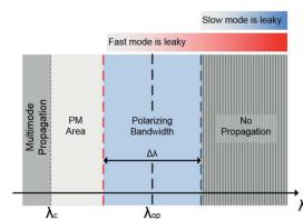
Transmission spectra showing two separate cut-offs for the polarization modes in the fast and slow axes.
