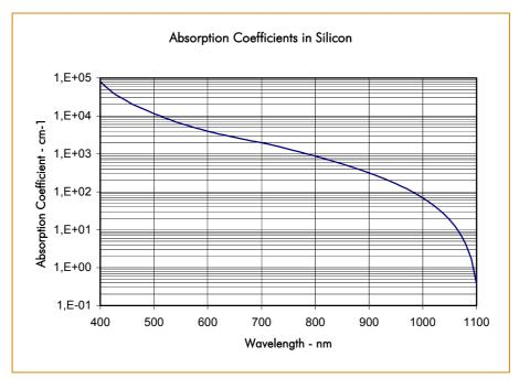
Figure 1. Absorption Coefficients in Silicon
