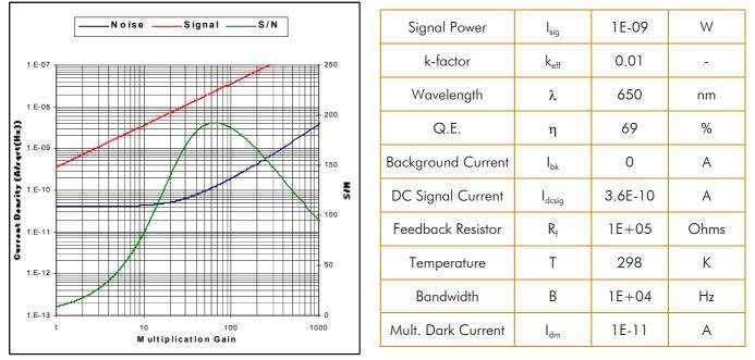
Figure 4. S/N Calculation. Low noise, High Optimum Gain
