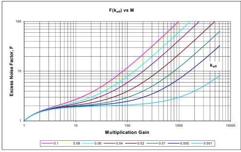
Figure 3. Excess Noise Factor in an APD as a function of  $k_{\mbox{\tiny eff}}$  and Gain
