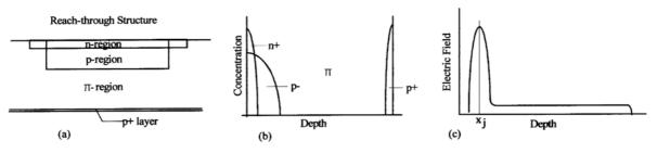
Figure 2. Silicon Reach-through APD Structure, Concentration and Field Profiles
